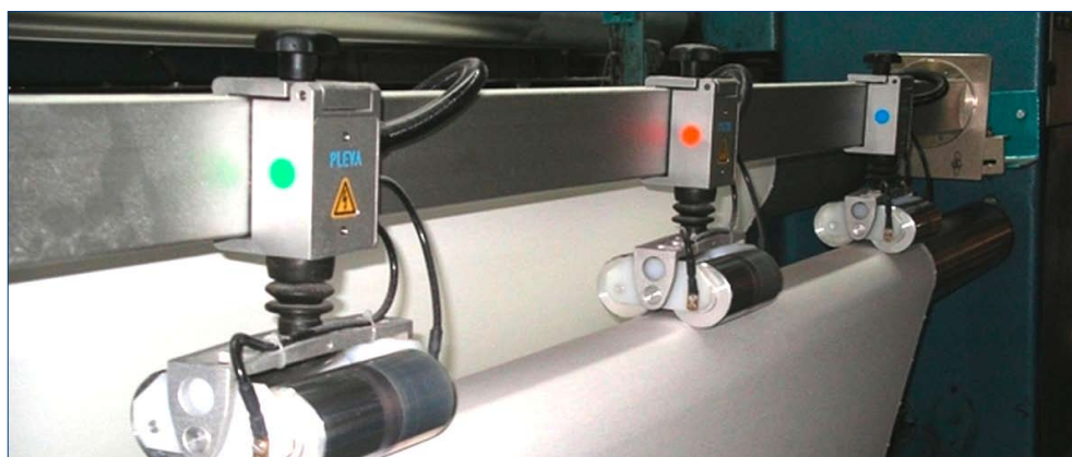
Sensor type RR 3.3 to measure over the width left - centre - right
