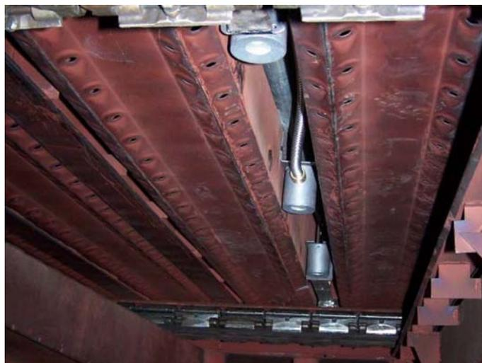
Fig. 9: TDS95 temperature sensors for profile side/centre/side retrofitted on an old Krantz stenter
