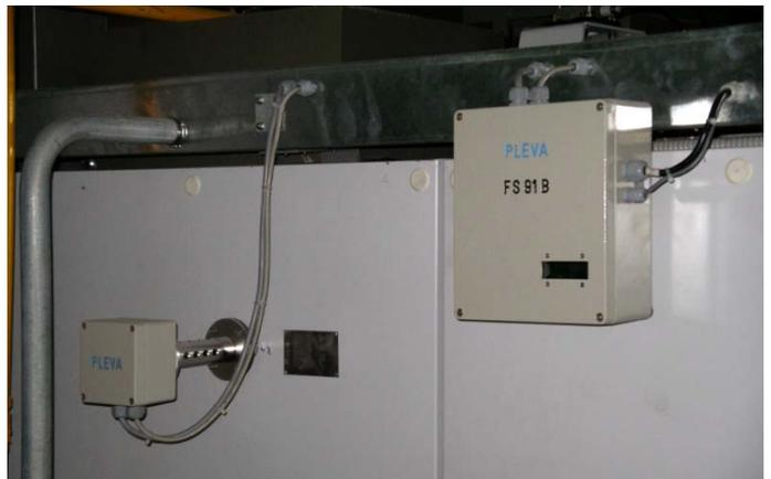
Fig. 3: Exhaust humidity measurement FS91 on stenter frame
