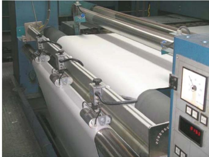
Fig. 5: Residual moisture measurement RR1.3 (side/centre/side)
