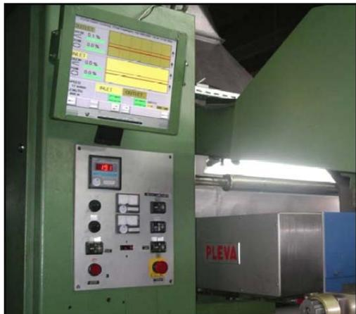
Fig. 15: Inlet/Outlet display of distortion on a stenter (Structure Detector SD1 traversing)
