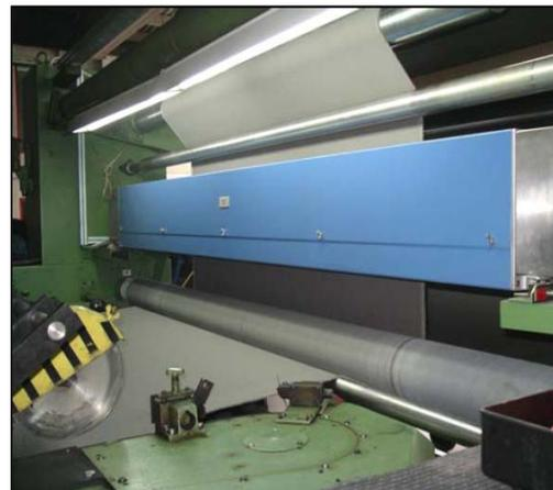
Fig. 16: Outlet reading bridge SD1 on a stenter (Structure Detector SD1 traversing)
