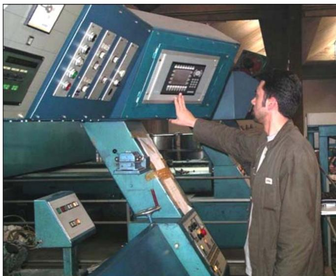
Fig. 1: HeatSet Control on Krantz stenter frame in DEBA Turkey.
