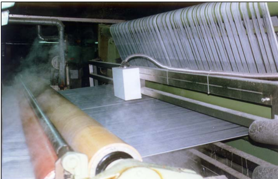
Fig. 1: Microwave measuring head PLEVA type AS120, protected against steam vapor behind the size box.
