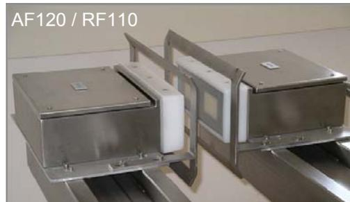
The standard coating paste is based on a defined ratio between water and solids. The water content is measured contact less, continuously and accurately by the microwave system. The amount of absorption of microwave is a measurement of the absolute moisture content and the coating addon. Reproducible adjustments are made with this reliable output signal.
