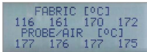
Depending on the weight / type of fabric and the thickness of the coating paste the surface temperature only is not sufficient enough for monitoring and control of drying / curing processes. Therefore the sensor shows two °C temperature information.
