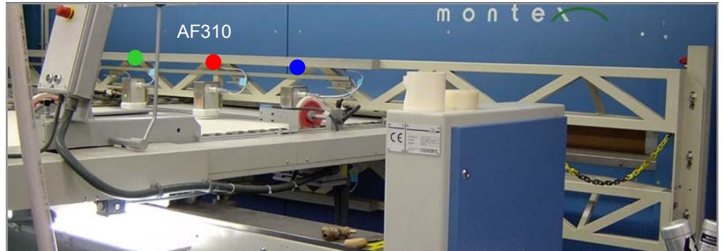
AF 310 installation directly after the coating head just in front of a coating stenter
