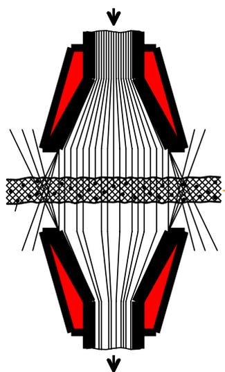
Measuring principle: Microwave absorption
