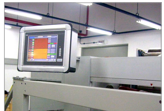
Picture 3: PlevaTec Touch operator panel with graphic screen and data storage in protective cabinet.
