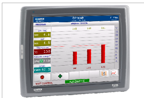
CIMATIC controller type PP70 OPTIDRY with Touch screen and colour graphic display 6.5" TFT. Trend graph, data storage and modular PLC unit, removable flash memory card.
