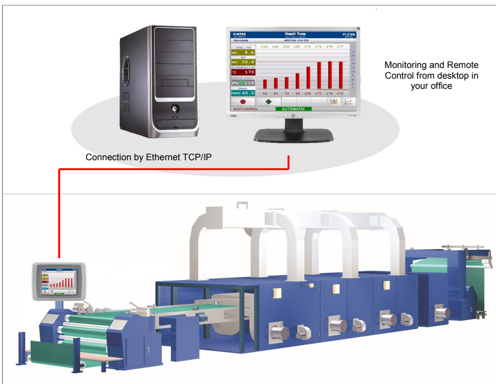
Stenter frame with CIMATIC control panel, connected to local network to supervise the process from the office
