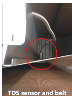
Tensionless relax dryer for open width knit goods with ECO-OPTIDRY control and required sensors
