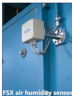
Tensionless relax dryer for open width knit goods with ECO-OPTIDRY control and required sensors
