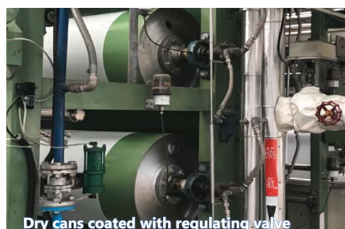
Dry cans coated with regulating valve
