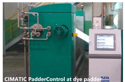
Microwave measurement AF 310 at dye padder
